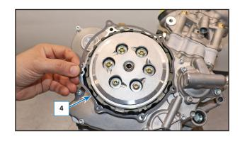
Mount the clutch guard (3) and tighten the screws (1) M5-L65 and (2) M5-L25 gradually with a torque of 8 Nm (0.8 kgm/ 5.9 ft/lb)
