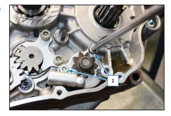
Remove the pump (2) by lifting it.
