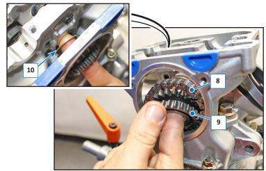
Correctly place the timing chain (8) on the drive gear (9).
