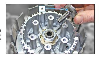
Remount the pressure plate (7) with the relative springs (6).
