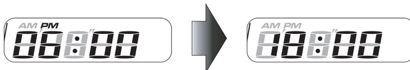
From the time home screen page, press the “Select” button from 3 seconds to change the clock display from 12 to 24 hour format or vice versa.
