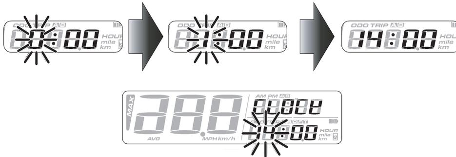
Press the “**Adjust**” button to move to the minutes setting. The following screen page is displayed:
