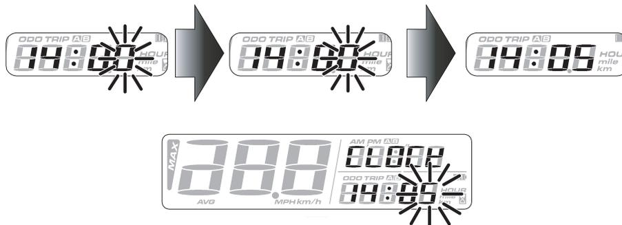
Press the “Adjust” button to return to the clock setting screen page:
