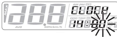
The minutes value flashes. To set the minutes, for example 5, press the “**Setup**” button as many times as needed to reach the desired number of minutes.
