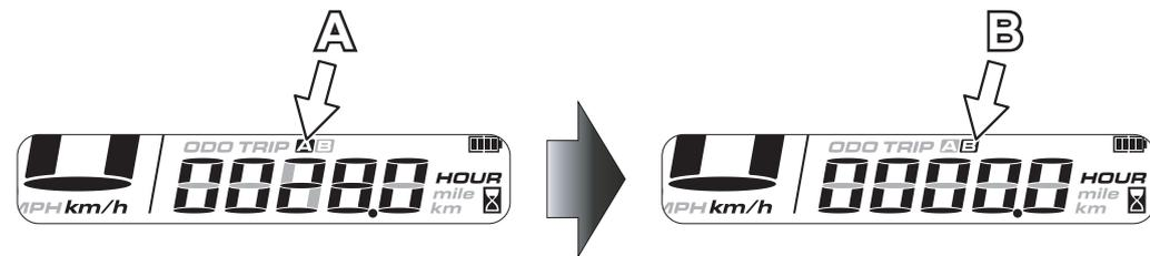
To reset the partial hours of operation both in “A” and in “B” with the function active press the “Adjust” button for three seconds.
