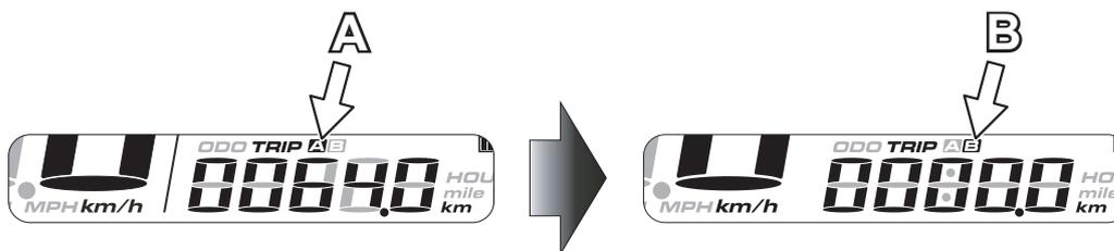
To reset the km/miles travelled both in “Trip A” and in “Trip B” with the function active press the “Adjust” button for three seconds
