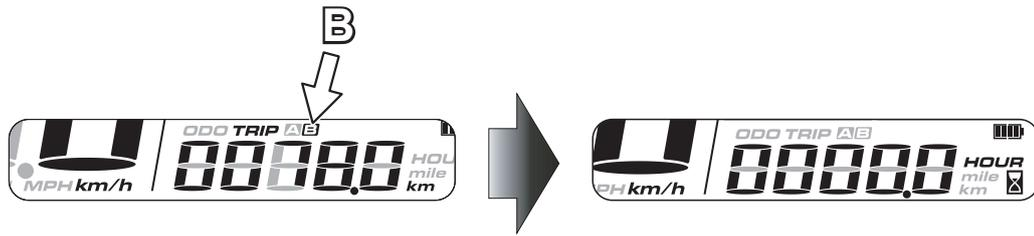
Press the “Adjust” button to switch from the total hours of engine operation to the partial hours of operation “A”.
