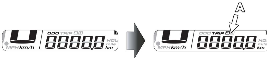
From “Trip A” press the “Adjust” button to go to the “Trip B” partial km/miles travelled function.
