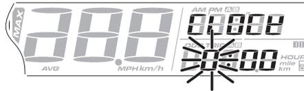
The hours value flashes. To set the hours, for example 14, press the “**Setup**” button as many times as needed to reach the desired hours number.
