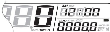
Starting on the home screen page, press the “Adjust” button once to switch from the odometer function (total km / miles travelled) to the “Trip A” partial km / miles travelled function.
