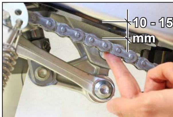
**TENSIONING THE CHAIN (EN/MX/SMR/SMX)**
