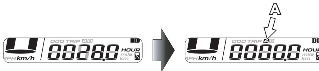
From “A” press the “Adjust” button to switch to the display of partial hours “B”.
