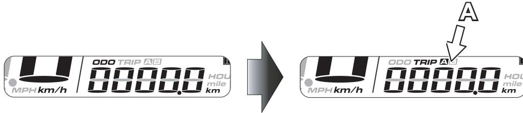
From “Trip A” press the “Adjust” button to go to the “Trip B” partial km/miles travelled function.
