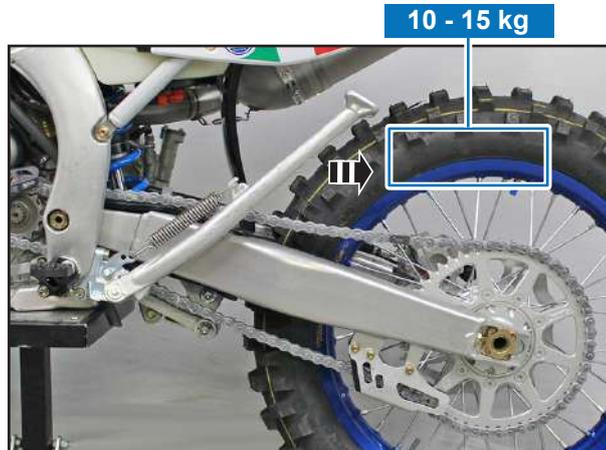
Chains do not wear evenly, therefore repeat the measurement in different points.
