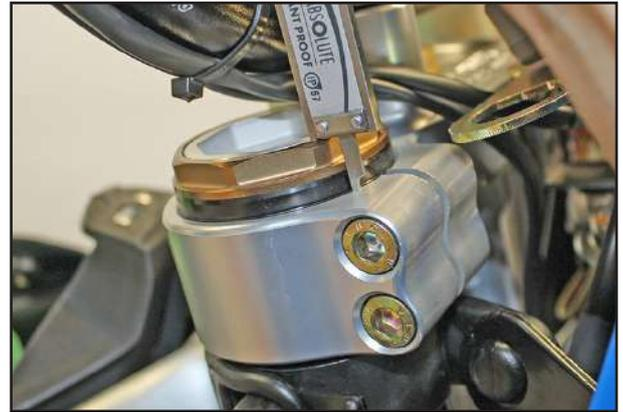
**NOTE:** Normally the distance is approx. 13 mm on the first reference notch of the rod.
