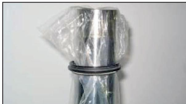
**NOTE:** Apply grease to the edge of the sealing ring.
