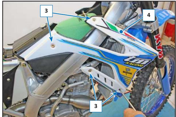
**NOTE:** On re-mounting, position the bushes correctly under the screws.
