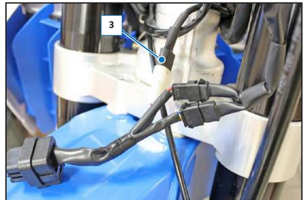
**NOTE:** On re-mounting, fix the cabling using plastic straps, as previously described.
